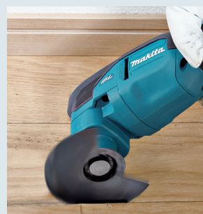
Cutout in the flooring
