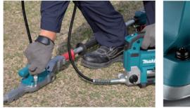
Users who do not own a grease gun can remove the bolt and supply grease with a grease tube as with our current models.
